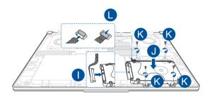
**NOTE:** The flexible printed circuit cable is bent in a particular shape. DO NOT try to change the original shape or press the fold line excessively.
